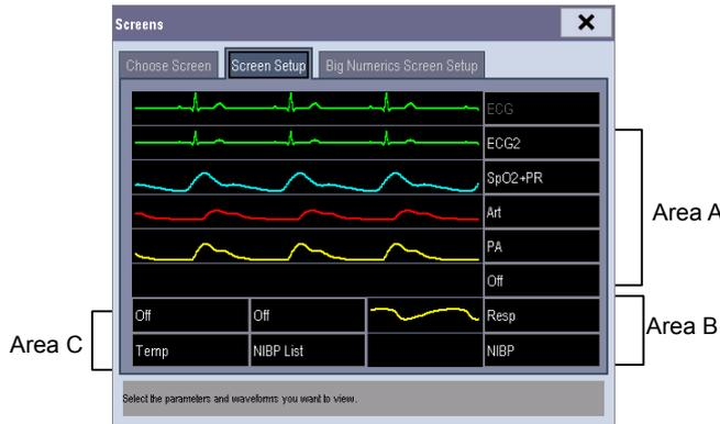
The ECG parameter and the first ECG waveform always display in the first row. The configurable areas can be classified as Area A, Area B, and Area C.
