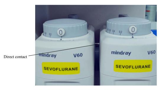
When the anesthetic delivery system has three and more than three groups of plug-in connectors, check if there is an interlock function between nonadjacent connectors. Otherwise, vaporizers are recommended to be connected right next to each other.
