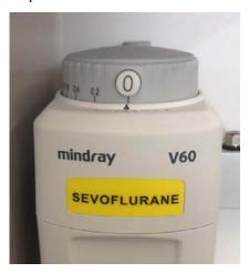
5. Hold the vaporizer in vertical position with both hands and lower gently onto the anesthesia machine plug-in connector.
