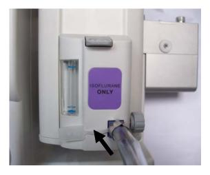
6. Tighten the lock knob clockwise.
