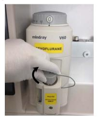
7. Tighten the cap of the anesthetic agent bottle even if it is completely empty.
