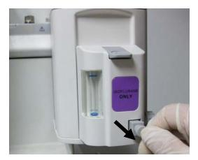
7. Push the keyed end of the filling adapter into the opening of the filling system until it cannot move.
