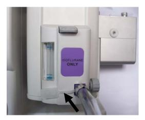
8. Tighten the lock knob clockwise.
