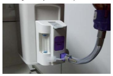
8. Open the filler control and the liquid agent will flow into the vaporizer.
