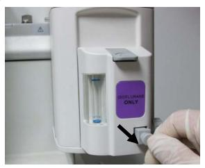
5. Push the keyed end of the filling adapter into the opening of the filling system until it cannot move.
