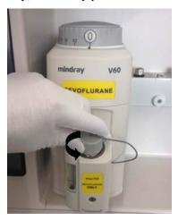
3. Check if the names of anesthetic agent and color mark on the vaporizer and the anesthetic agent bottle correspond. If the correct agent is being used, unscrew the cap from the anesthetic agent bottle. Pour anesthetic agent slowly into the filler receiver.
